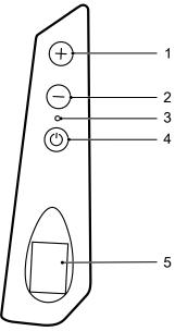
Fig. 13: Buttons and display at the frequency inverter
