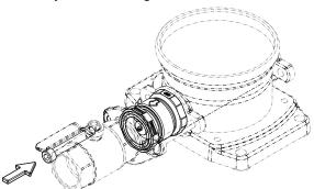
Fig. 21: Fitting the screw
