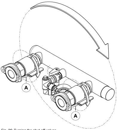
Fig. 26: Turning the shut-off valves
