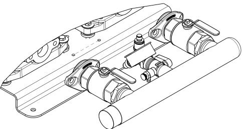
Fig. 23: Removing the manifold
