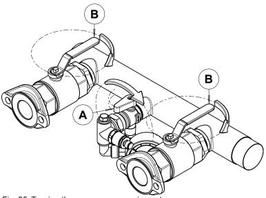
Fig. 25: Turning the pressure measuring set
