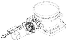
Fig. 15: Removing the screw
