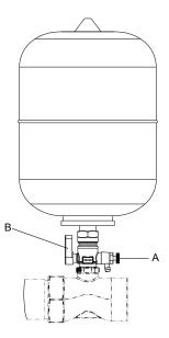
Fig. 12: Venting and draining the accumulator
