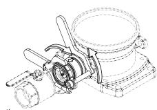
Fig. 16: Screwing the valve's body parts into each other
