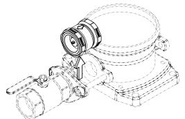
Fig. 17: Removing the body
