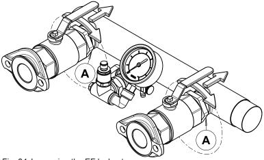
Fig. 24: Loosening the EF locknut
