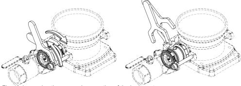
Fig. 19: Loosening the screwed connection of the body parts
