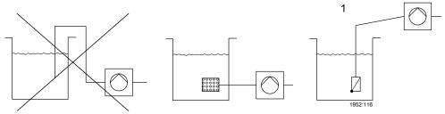
Fig. 10: Correct piping connection
