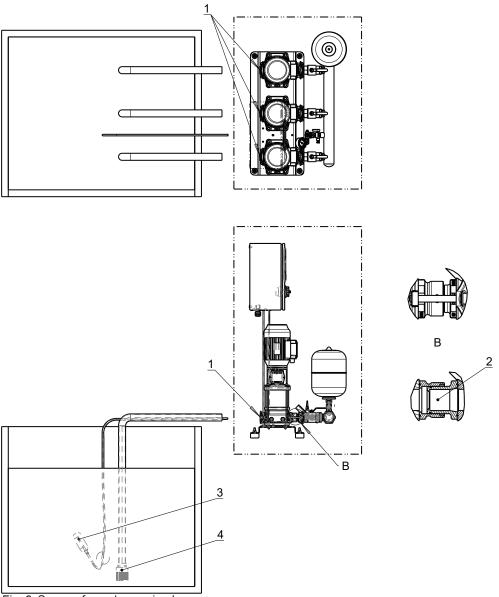
Fig. 8: Scope of supply, version L
