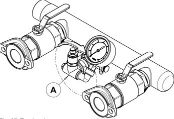
Fig. 27: Turning the pressure measuring set
