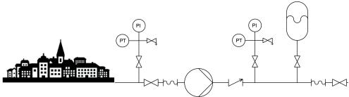
Fig. 3: M = Inlet side of pressure booster system connected to the municipal water supply, suction head operation
